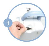
Connect your Inogen One AC Power Supply cord to the AC Power Supply. Connect the AC Power Supply to your Inogen One.
