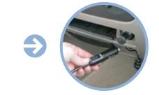
Plug the mobile power charger into the cigarette lighter or auxiliary DC power supply.
