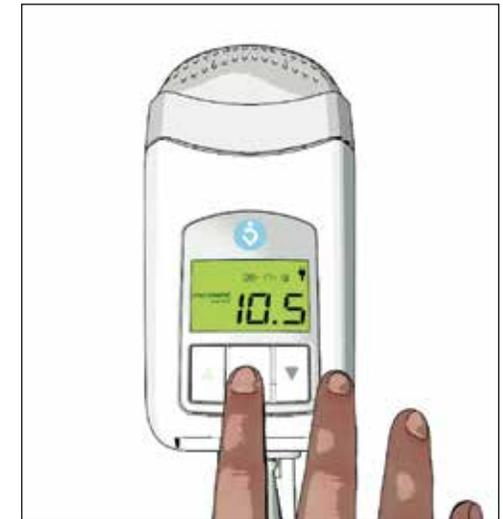
**IMPORTANT:** The "REMINDER" indicator will display on the Z1 if an air leak is detected between the Z1 outlet and the mask. This may also display at times when the mask is not being worn properly. This common condition should clear once all connections are secure, the mask is properly worn, and therapy has begun.
