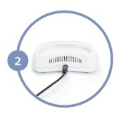
Plug the External Battery Charger AC power supply into the battery charger.
