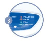
An illuminated red light on the left of the charger indicates the power is on.
