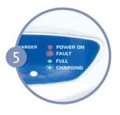
When the battery is in the correct position, a flashing green light will indicate that the battery is charging. When the green light stops flashing the battery is fully charged.\*
